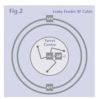
Interference is also major concern in such an environment. Multipath RF effects caused by the reflective metal surfaces from the vessel and pipes and background RF noise caused by large electrical machinery such as DC motors etc needs to be taken into account, otherwise a reliable connection will not be possible. The 5 GHz band was chosen as there is normally less background noise in this spectrum and it also leaves the 2.4GHz band free for a WiFi network to be installed at a later date.
