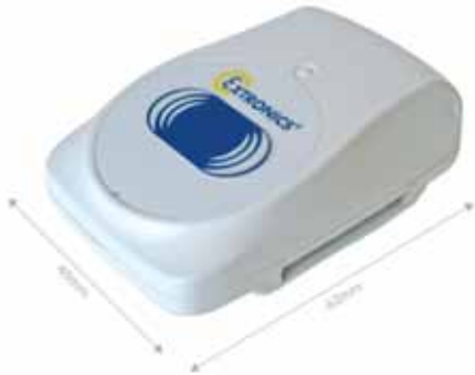
Figure 2. iTAG100 Active WiFi &amp; LF RFID Tag
