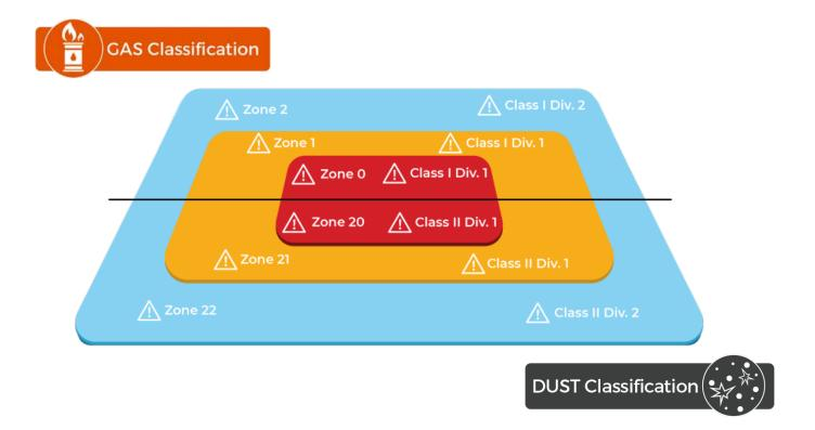
Figure 1: Different flammable gas and dust classification
