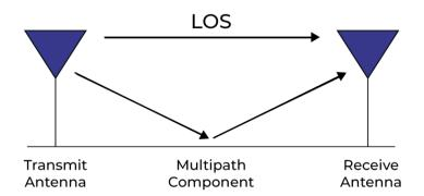
Figure 7: multipath interference diagram
